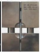
This arrangement helps when testing high stiffness materials like ceramics infused polymers, where the number and severity of flaws under maximum stress is directly related to the flexural strength and crack initiation in the material. Compared to the three-point bending flexural test, there are no shear forces in the four-point bending flexural test in the area between the two loading pins.
