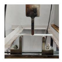
For most composite materials, the compressive strength is lower than the tensile and the specimen will fail at the compression surface. This compressive failure is associated with the local buckling (micro buckling) of individual fibres.
