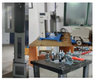
7. Heat Deflection Temperature: The heat deflection temperature of a reinforced or unreinforced polymer material is a measure of polymer's resistance to distortion under an applied load at elevated temperatures. The test specification for the HDT is <u>ASTM D 648</u> and ISO 75. HDT tests typically test for the short term performance of the materials under loads at elevated temperatures.
